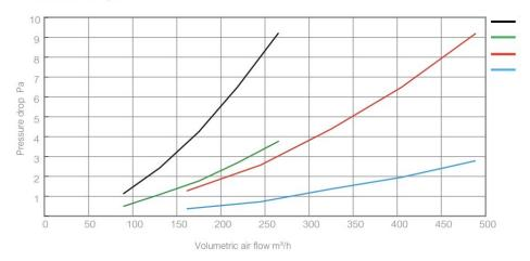
Bend 90° 160/125 insulated Duct 160/125 Bend 90° 200/170 insulated Duct 200/170
