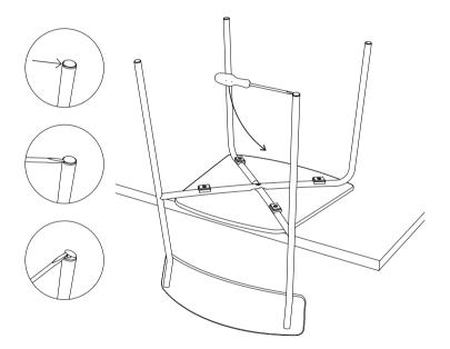
You can later exchange the glider by placing screwdriver in groove and push down
