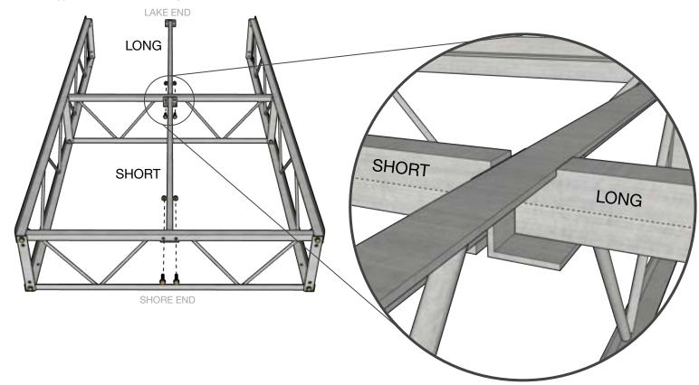
4 Attach Connecting Rail (0) to Side Rails and Long Center Support Tube. Use
