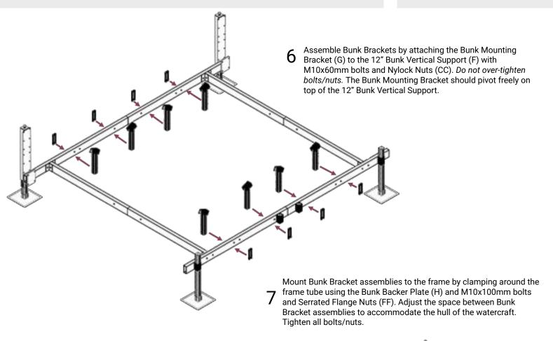
Screw wood bunks (not included) to Bunk Mounting Brackets (G) using two pan head screws (GG). To install, lay out wood bunks on assembled lift. Screw bunks into the Bunk Mounting Bracket.
