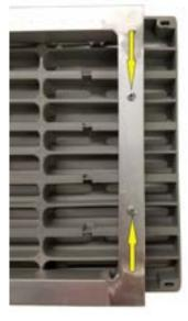
**Poly**: Align Aluminum Bench Frame (B) to pre-drilled holes on the bottom side of the Poly board using included M4x40mm Pan Head Screws (DD). Secure each Frame with (6) screws.
