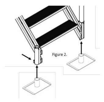
2 Insert Drop Leg and Base (C) into the bottom of each Stair Stringer (A). Find your desired height and tighten the pinch bolt on the Stair Stringer Bracket. See image to the left for a reference.
