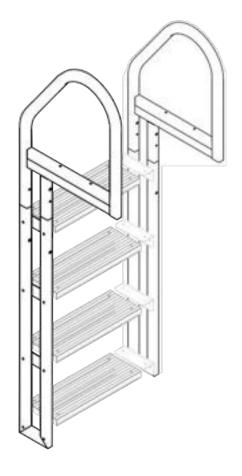
The Step Boards (C) will sleeve over the Step Bracket (D) and are fastened using two M6x20mm bolts/nuts (AA) on each side of the Step Board. Attach each Step Board to one of the Side Frame assemblies then position the second Side Frame assembly inside the Step Boards, tighten all bolts/nuts to complete assembly.
