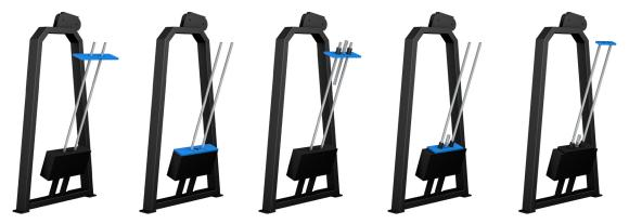
3.THE NUMBER OF INSTRUMENTS WITH SINGLE PIECE WEIGHT OF 10LB AND COUNTERWEIGHT OF 200LB IS 19 + 1(HEAD PIECE).
