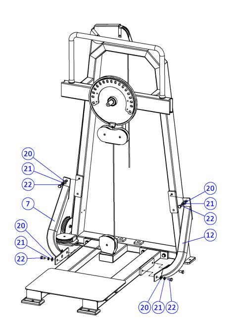
**STEP 3:** INSTALL THE GUIDE ROD, COUNTERWEIGHT, ETC., AND ATTACH THE STEEL WIRE THE ROPE IS STRUNG INTO THE PULLEY AND INSTALLED ON THE LOCK HEAD OF THE ADJUSTING LEVER OF THE COUNTERWEIGHT PLATE, AND THE ROPE IS INSERTED INTO
