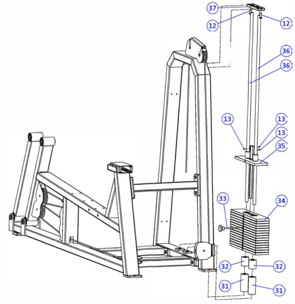
**STEP 3:** INSTALL INNER AND OUTER GUARD PLATES AND PLASTIC PULLEY COVER TO TOP OF WEIGHT STACK FRAME.
