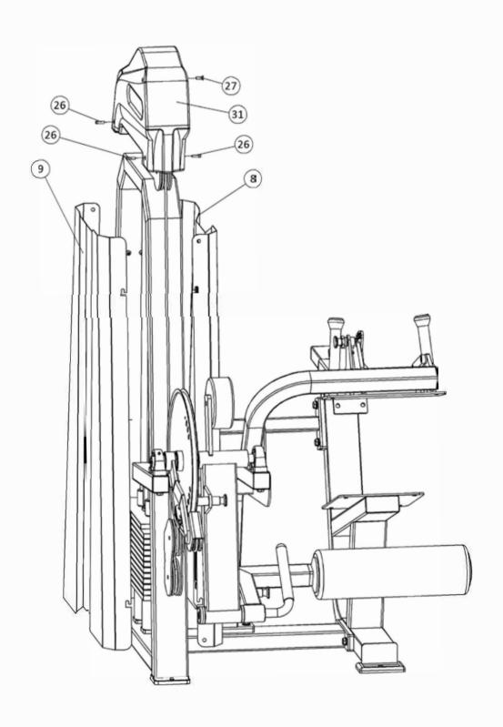
**STEP 6:** INSTALL BACK CUSHION, LEG CUSHION, SEAT CUSHION, TIGHTEN SCREWS.
