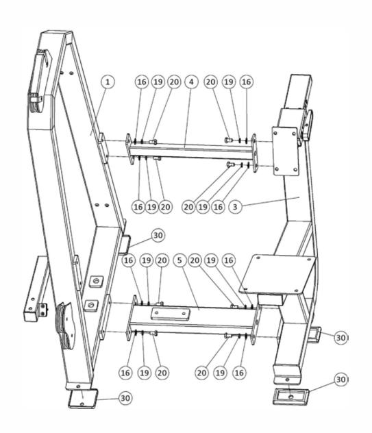
**STEP 2:** INSTALL THE ADJUSTABLE QUADRICEP SUPPORT (2) TO THE WEIGHT STACK FRAME AND BOTTOM BASE ATTACHMENT AS SHOWN IN THE DIAGRAM.
