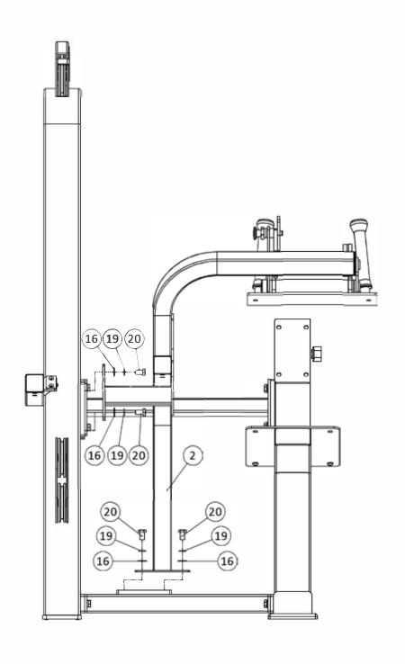
STEP 3: INSTALL THE ADJUSTABLE CAM ASSEMBLY TO THE WEIGHT STACK FRAME BY ATTACHING TO TWO PILLOW BLOCK BEARINGS AND 4 BOLTS. TAKE OUT THE WEIGHT STACK CABLE FROM THE ADJUSTABLE CAM ASSEMBLY AND PASS BETWEEN THE TWO PULLEY'S BELOW THE LARGE CAM. THEN THE CABLE TO THE TOP PULLEYS ABOVE THE WEIGHT STACK. FEED THE CABLE THROUGH THE HOLE AFTER STEP 4 IS COMPLETE. INSTALL THE LONG FOAM ANKLE PAD (10) AND STEEL ADJUSTABLE ANKLE ASSEMBLY THAT PAD (10) CONNNECTS TO.
