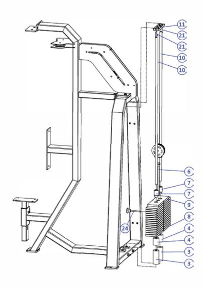
**STEP 3:** INSTALL THE ARMS(2) AS SHOWN IN DIAGRAM USING #14 AND #15 BOLTS TO THE MAIN FRAME ASSEMBLY. LOOP THE CABLE STARTING ON THE CAM CONTAINING SELECTOR HOLES DOWN AND AROUND THE PULLEY ATTACHED TO THE TOP PLATE AND BACK TO THE OPPOSITE CAM CONTAINING THE SELECTOR HOLES.
