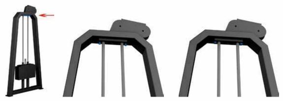
5. FIRST MOVE THE PLASTIC FIXING PLATE TO THE POSITION SHOWN IN THE FIGURE, AND THEN TIGHTEN IT WITH SCREWS TO COMPLETE THE WHOLE INSTALLATION PROCESS OF COUNTERWEIGHT PIECE.
