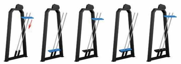
1. INSERT THE FIRST COUNTERWEIGHT PIECE FROM TOP TO BOTTOM.
