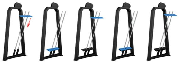
1. INSERT THE FIRST COUNTERWEIGHT PIECE FROM TOP TO BOTTOM.
