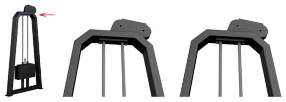
FIRST MOVE THE PLASTIC FIXING PLATE TO THE POSITION SHOWN IN THE FIGURE, AND THEN TIGHTEN IT WITH SCREWS TO COMPLETE THE WHOLE INSTALLATION PROCESS OF COUNTERWEIGHT PIECE.
