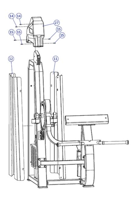
STEP 5: INSTALL ELBOW PADS AND SEAT CUSHIONS.
