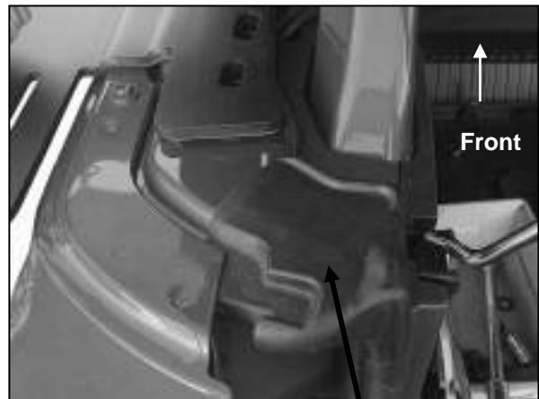
(Fig 16) Place the driver/left Mounting Bracket in place over threaded holes in body. Remove backing and apply adhesive backed Foam Rear Seal (see Fig 17) to top of body, between top and body
