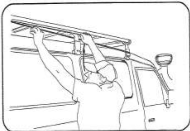
Secure strap provided to your roofrack or bars and then adjust one end by pulling on strap.
