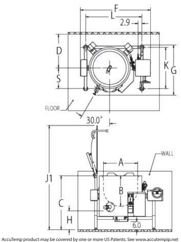
\*Dimensions on these drawings are applicable when using an optional 2" diameter draw-off valve. If a 3" diameter draw-off valve is required, contact AccuTemp for applicable dimensions.
