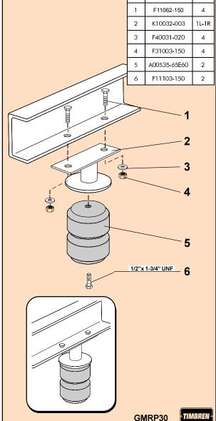
Do not exceed vehicle manufacturer's recommended axle weight rating. Check for AEON® interference with vehicle components - Under load AEON® will "expand" in diameter.
