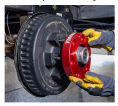
4. Install supplied lug nuts. Tighten until snug on crisscross pattern. Using another set of wrench, hold hub to prevent it from turning. Torque lug nuts in crisscross pattern to 100-110 ft-lbs.
