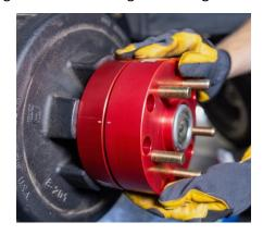
8. Install 6 supplied Socket Head Cap Screws using 1/4" Allen key.
