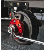
5. Pre-Assemble 5 supplied lug bolts to Part B as shown. Torque them to 70-90 ft-lbs.
