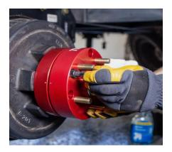
9. Using another set of wrench, hold hub to prevent it from turning. Torque cap screws in crisscross pattern to 90-100 ft-lbs.
