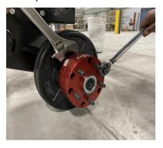
10. Install Jeep wheels. Ensure rim has between 35mm to 44.45mm positive offset.
