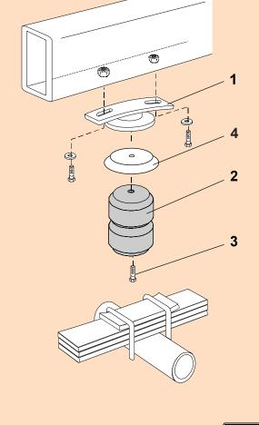
Do not exceed vehicle manufacturer's recommended axle weight rating. Check for AEON® interference with vehicle components - Under load AEON® will "expand" in diameter.
