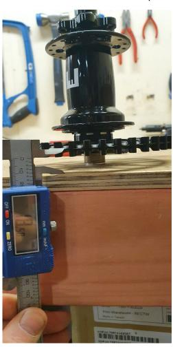
Or is can be checked on the bike by measuring the distance between the inside of the rear belt guide and the centre line of the rear cog
