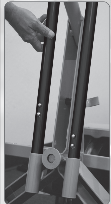
Storing front legs in travel socket
