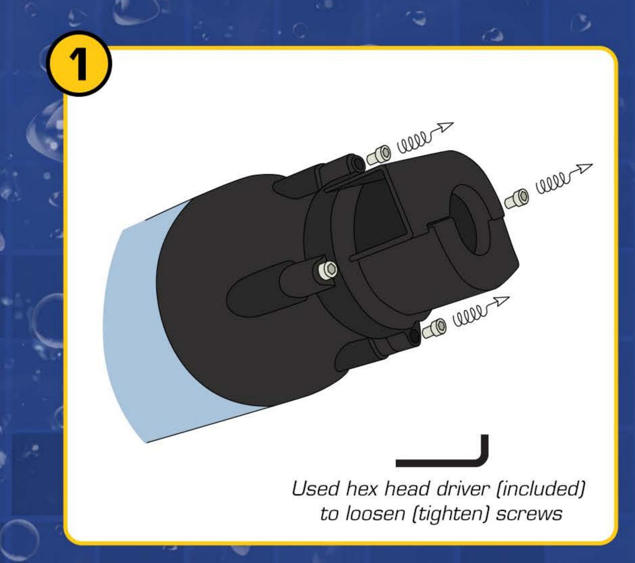
Remove 4 hex head screws and remove the diffuser cap. Carefully set screws and washers aside.
