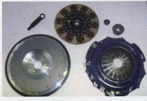
▲ High rpm isn't all about the valvetrain and intake; you need a lightweight clutch and flywheel to let the engine rev freely. The setup must offer enough grip to put more than 600 lb-ft to the ground. As such, Rick commissioned AFM's own line of Hi-Rev clutches designed to allow shifting as high as 7,600 rpm without the pedal sticking to the floor. For his car, Rick opted for Stage III unit (\$550) and one of AFM's Superlight flywheels (\$329), which is 14 pounds lighter than a stock flywheel.
