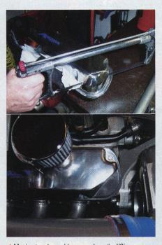
▲ Moving to a larger blower such as the YSi means you're bound to have some bumps in the road. It became clear that Rick's pretty valve covers wouldn't allow his experimental 5-inch Power Pipe fit on the blower's inlet—the standard 4-inch Power Pipe fits fine. As such, Rick did some customizing with a hacksaw and a welder. This trick didn't interfere with the rocker arms and left plenty of room for the 5-inch Power Pipe.
