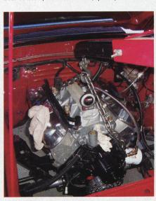
▲ Finally, Rick is ready to drop the engine in place. Unlike most of us, he actually takes the time to use a level to ensure the motor goes in straight. We're not sure if Rick is just a stickler for right angles or if he's trying to eek out that last horsepower by reducing driveline bind. Maybe he's just trying to freak us out.
