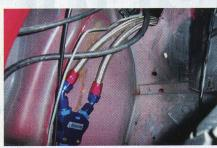
▲ As is typical of big fuel-system installs on Fox Mustangs, Rick mounted a Y-block inside the passengerside inner fender, then routed the lines to the fuel rails, and on to the regulator. This monster fuel system feeds eight Delphi 85-lb/hr injectors (\$565), which proved easily up to the task of fueling the pump-gas combo. The injectors get the proper instructions from the PMS, thanks to a like-calibrated mass air meter from PMAS (\$449).
