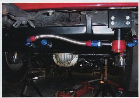
▲You'll have to provide your own sumped tank to properly set up this type of system. Rick couldn't speak highly enough about this fuel pump, saying it delivered 160 gallons per hour through 16 feet of fuel line, even at 60 psi. That's a lot of flow. Another reason he chose the pump was its compatibility with alcohol—thus E85, should he wish to try alternative fuel testing.
