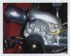
▲ Rick puts AFM Power Pipes on all his cars, but they don't all get rigidly mounted YSi-Trim superchargers driven by cog belts. This setup is only for cars that Rick wants to drive to work.
