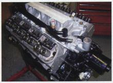
▲ With TDC confirmed, Rick installed his Trick Flow Twisted Wedge heads featuring AFM Stage III porting (\$2,388). These are the standard TW heads with healthy porting—no race heads here. Remember, this is a street car. The lower intake also in place is a Trick Flow R lower, which Rick will top with a Vortech Mondo Box upper intake. That package goes for \$788, but it supports big power.
