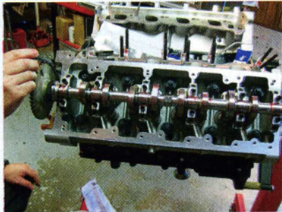
▲ For the move from the stock engine's flat-top pistons to the supercharger-compliant, dished slugs in the SuperMOD stroker, AFM's N-22 camshaft had to be replaced with a pair of N-52 bumpsticks. The new cams are designed to work well in engines with aftermarket pistons, and Trick Flow or ported PI heads. The N-52s are healthy and don't like driving under 2,400 rpm, according to Rick Anderson. As the cams' rev range (3,500-7,200) is about 1,000-rpm higher than that of the N-22 camshafts (2,400-6,200 rpm), 4.30 or even 4.57 gears are perfect for great street performance with this type of engine.
