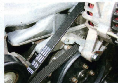
▲ Trick Flow's 4.6-liter Track Heat intake manifold is being used for the new engine setup, so the alternator must be installed backward (turned around so the pulley faces the firewall) to achieve proper serpentine-belt alignment. This is where the engine swap's only modification happens. By slightly cutting and grinding on Trick Flow's alternator bracket Nikki's crew is able to achieve enough clearance for the belt as it travels across the larger ASP water-pump pulley.
