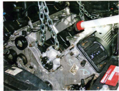
▲ The new D.S.S. powerplant is lowered between the fenders of Nikki's '02 ragtop. Once the engine is secured on the K-member and mated with the tranny, all of the accessories, pulleys, exhaust and other reused pieces (that were disconnected for the original engine's extraction), are now bolted in place.
