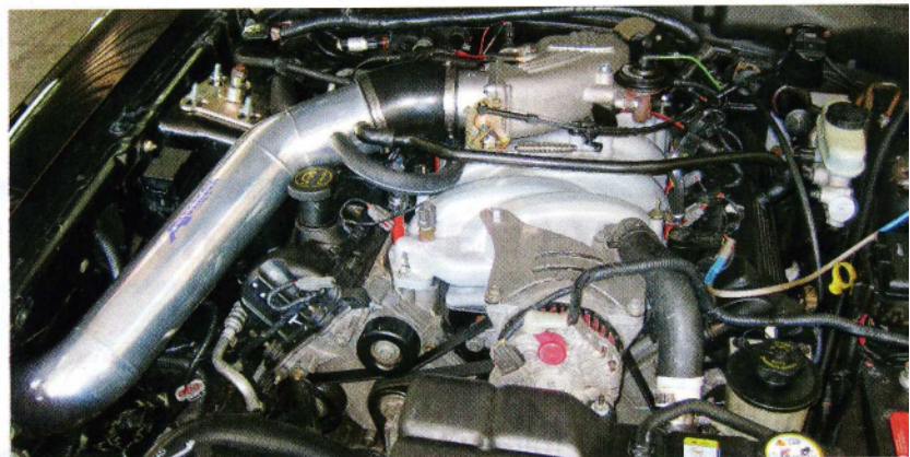
▲ The D.S.S. 5.0 SuperMOD is completely installed and ready to rock in Nikki's '02 GT. In addition to the aforementioned Trick Flow Track Heat intake (PN TFS-51900002-M44), a Professional Products (www.professional-products.com) 75mm throttle body (PN PP-69223) and Ford Racing Performance Parts' 30-lb/hr fuel injectors (PN M-9593-BB302) have been added as completion parts for the new mill. We're interested in seeing how the manifold works on this naturally aspirated setup. The intake's symmetrical port and the 75mm throttle body should generate a substantial increase and even distribution of airflow to each cylinder. 5.0
