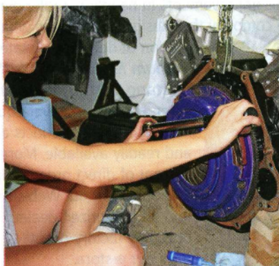
▲ Anderson's Stage I Hi-Rev clutch system (PN KITHRC1A-468) is Nikki's choice for ensuring smooth engagement of her five-speed's gears. The clutch is designed for supercharged engines that rev through 7,500 rpm, and it features a 10.5-inch organic clutch disc and AFM's Super Light eight-bolt (SFI rated) flywheel. The significant weight difference between the factory flywheel and Anderson's SFI-rated 'wheel definitely will have a big impact on the GT's quick acceleration once the blower is installed.
