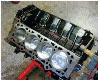
▲ Nikki selected a D.S.S. 5.0 SuperMOD short-block as her Pony's new motivator. The short-block features D.S.S.' Extreme-X forged dished pistons (9.6:1 compression); a KPC micro-alloy forged, 3.750-inch crankshaft (eight-bolt); 5.850-inch forged-steel, H-beam rods; and a D.S.S. Pro Mod Main Support System, which, along with ARP main studs, will keep bottom-end harmonics stable at high rpm.
