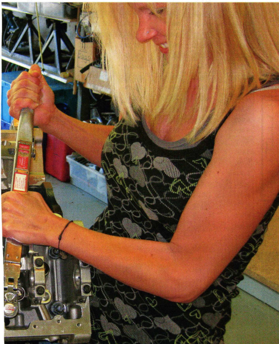
▲ Nikki selected a D.S.S. 5.0 SuperMOD short-block as her Pony's new motivator. The short-block features D.S.S.' Extreme-X forged dished pistons (9.6:1 compression); a KPC micro-alloy forged, 3.750-inch crankshaft (eight-bolt); 5.850-inch forged-steel, H-beam rods; and a D.S.S. Pro Mod Main Support System, which, along with ARP main studs, will keep bottom-end harmonics stable at high rpm.
