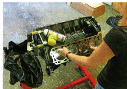
▲ Nikki uses a clean rag and a little oil to give each cylinder in the Level-10-prepped short-block a final cleaning and a small amount of lubrication before final assembly begins.
