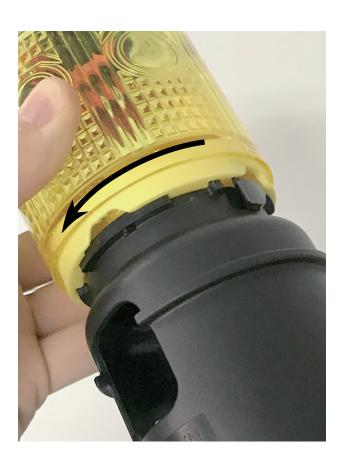
Remove: Using thumb, push tab in below the LED light. With tab pushed in, twist LED light clockwise to unlock and remove.
