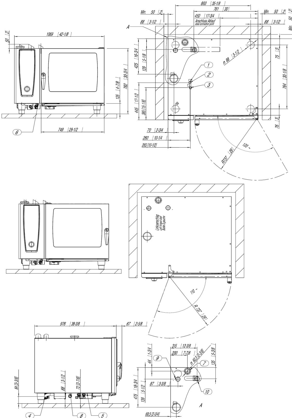
1. Common water supply (cold water) "Single" water connection as shipped
