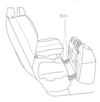
(1996-02) 12mm bolt | rear/bottom seat | passenger side (2003-24) 14mm bolt | rear/bottom double-seat | depends on trim
