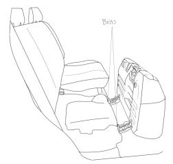
(1996-02) 12mm bolt | rear/bottom seat | passenger side (2003-24) 14mm bolt | rear/bottom double-seat | depends on trim
