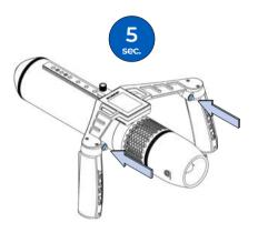
2 Turn the SCUBAJET on/off by pressing the 2 buttons on the Dual Hand Controller for 5 seconds.
