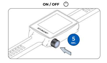
1 To turn on/off the remote control, press the button for 5 seconds.
