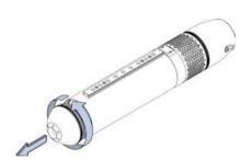
1 Rotate the nose counter-clockwise to open the SCUBAJET.
