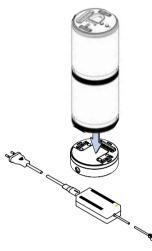
Put the batteries in a vertical position on the charger for easy handling.
