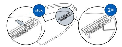
**1A Slide-In Finbox:** No screws are necessary for the Slide-In Finbox. The clip must engage.
