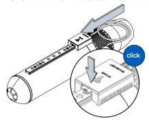
Attach the BT-Link SSC connector to the SCUBAJET accessory rail by holding the SCUBAJET upside down. Wait until the SCUBAJET logo on the BT-receiver starts blinking. This means that the device is ready for Bluetooth pairing.
