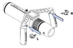
**3** Press the right button to speed up or the left button to slow down.
