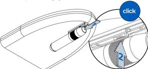
**2** Make sure the SCUBAJET does not extend over the edge of the SUP board.
