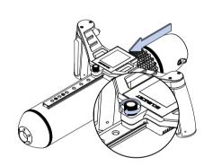
1 Securely attach the Dual Hand Controller to the adapter rail on the tube, tightening the screw clockwise until it is firmly in place.
