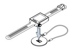
Place the remote in the middle of the charger until the light changes from red to blue. The remote begins charging only when the light turns blue. The display will show you when the remote is fully charged.
