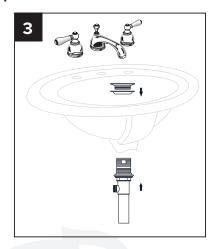
Mount the drain assembly and faucet (not included) on the sink, following faucet manufacturer's instructions. Be certain to apply a bead of sealing putty on the underside of the drain in order to ensure a watertight seal between the sink and drain. Remove excess putty after installing drain on sink.
