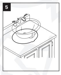
Center bowl and install. Remove excess sealant from inside lip.
