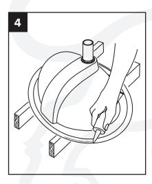
After checking fit and alignment of sink to cut out, apply a bead of silicone adhesive to rim of sink. NOTE: Do not use other construction adhesives or adhesive sealants.
