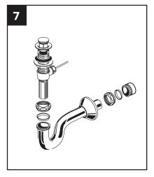
Connect trap to drain assembly hand tight to check alignment. It may be necessary to cut off part of the tailpiece or part of the horizontal leg of the trap. Secure joints for watertight assembly.
