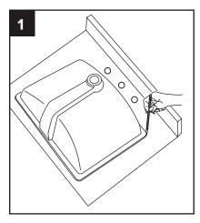
First, make sure the clearance between the backsplash, faucet, fixtures and cabinets are acceptable for the new sink. NOTE: To avoid damage to countertop, install sink such that future removal from underneath the countertop is possible.
