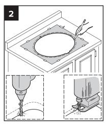
Carefully cut out the enclosed template, then position and trace the template on the countertop as shown on the template. Make a mark of the faucet hole centerline on the countertop. Drill a 1/2" pilot hole on the inside of the cut line. Use a saber saw or a keyhole saw to cut out the countertop opening.
