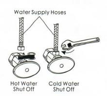
7. After installing the faucet, remove spray head (#4) from the hose (#3) and then turn on the hot and cold water shut offs. Check for leaks. If it leaks at the supply line connections at the faucet, please refer to step 6 for tightening procedure.
