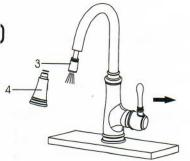
8. Turn on the faucet for one minute to flush the debris from the faucet. Turn off the faucet and reassemble the pull-down faucet spray head (#4) to hose (#3).
