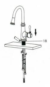
3. Attach spacer (#39)(if the thickness of counter top is less than 1/5"; if the thickness of counter top is more than 1/5", spacer (#39) is not needed), gasket assembly (#22) and lock nut (#23) from the bottom. Please Note: Please assemble in numerical order. Tighten but do not over tighten. Use a phillips screwdriver to tighten the 3-screws (#24) on the lock nut (#23). See diagram for visual.
