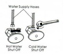
7. After installing the faucet, remove spray head (#4) from the hose (#3) and then turn on the hot and cold water shut offs. Check for leaks. If it leaks at the supply line connections at the faucet, please refer to step 6 for tightening procedure.
