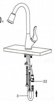
5. Attach the weight (#26) to the lowest point on the downward side of the hose (#3) to prevent the hose (#3) from twisting. The weight can be installed facing either direction, it will not move once tightened down.
