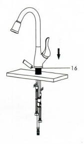
3. Attach spacer (#28)(if the thickness of counter top is less than 1/5"; if the thickness of counter top is more than 1/5", spacer (#28) is not needed), gasket assembly (#23) and lock nut (#24) from the bottom. Please Note: Please assemble in numerical order. Tighten but do not over tighten. Use a phillips screwdriver to tighten the 3-screws (#25) on the lock nut (#24). See diagram for visual.
