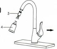
Turn on the faucet for one minute to flush the debris from the faucet. Turn off the faucet and reassemble the pull-down faucet spray head (#4) to hose (#3).
