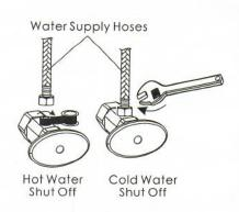
7. After installing the faucet, remove spray head (#9) from the hose (#8) and then turn on the hot and cold water shut offs. Check for leaks. If it leaks at the supply line connections at the faucet, please refer to step 6 for tightening procedure.
