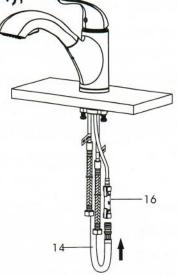
5. Attach the weight (#31) to the lowest point on the downward side of the hose (#14) to prevent the hose (#14) from twisting. The weight can be installed facing either direction, it will not move once tightened down.
