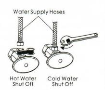
7. After installing the faucet, remove spray head (#9) from the hose (#8) and then turn on the hot and cold water shut offs. Check for leaks. If it leaks at the supply line connections at the faucet, please refer to step 6 for tightening procedure.
