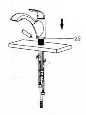
3. Attach spacer (#32)(if the thickness of counter top is less than 1/5"; if the thickness of counter top is more than 1/5", spacer (#32) is not needed), gasket assembly (#25) and lock nut (#26) from the bottom. Please Note: Please assemble in numerical order. Tighten but do not over tighten. Use a phillips screwdriver to tighten the 3-screws (#27) on the lock nut (#26). See diagram for visual.
