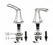
5. Place silicone sealant beneath the handle flange (#4) and install through the far left hole (hot water side), repeat the same process for the right hole (cold water side). See diagram for visual. From underneath the sink, re-assemble gasket assembly (#10) and lock nut (#11). Hand tighten lock nut (#11).
