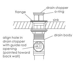
9. Remove rod guide nut and rod ball plastic gasket. Insert horizontal rod into drain body and through hole in drain stopper. Replace rod guide nut with rod ball plastic gasket and tighten it.
