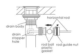
10. Place one end of the spring clip on the end of the horizontal rod. insert the ball rod through a hole on the lift rod strap, then slide the other end of the spring clip over the horizontal rod. See diagram for visual. Hint - Be sure to move the ball rod up and down a few times to make sure the drain stopper opens and closes before going to the next step.
