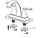
5. Connect the supply lines to the faucet and secure the nuts by adjustable wrench. The hot water supply should go on the left while the cold water supply should go on the right.
