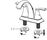
3. Place silicone sealant beneath the gasket (#10) and install faucet lines through the hole. See diagram for visual. (This faucet fits 3cm countertop.)
