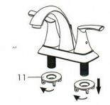
3.Place silicone sealant beneath the gasket (#10) and install faucet lines through the hole. See diagram for visual. (This faucet fits 3cm countertop.)
