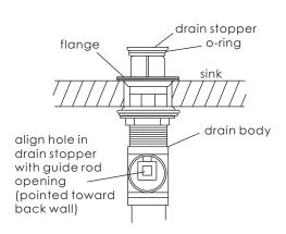
8. Remove rod guide nut and rod ball plastic gasket. Insert horizontal rod into drain body and through hole in drain stopper. Replace rod guide nut with rod ball plastic gasket and tighten it.
