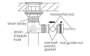
9. Place one end of the spring clip on the end of the horizontal rod. insert the ball rod through a hole on the lift rod strap, then slide the other end of the spring clip over the horizontal rod. See diagram for visual. Hint - Be sure to move the ball rod up and down a few times to make sure the drain stopper opens and closes before going to the next step.
