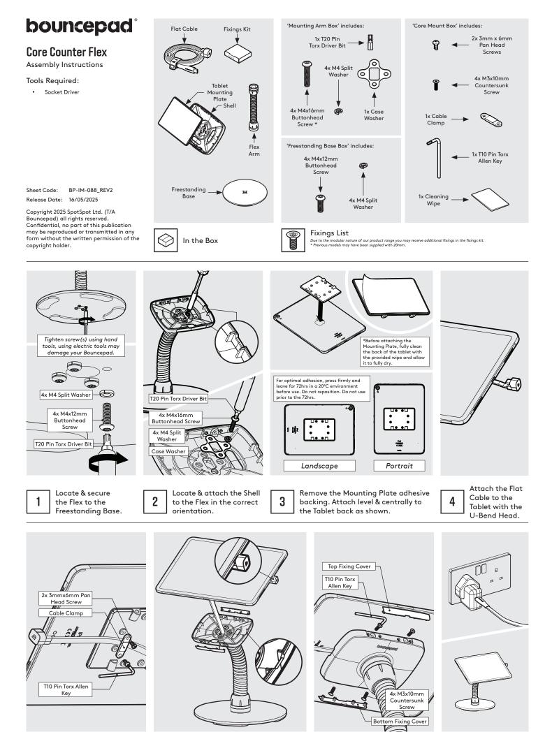
Secure the Flat Cable to the Mounting Plate with the Cable Clamp as shown.
