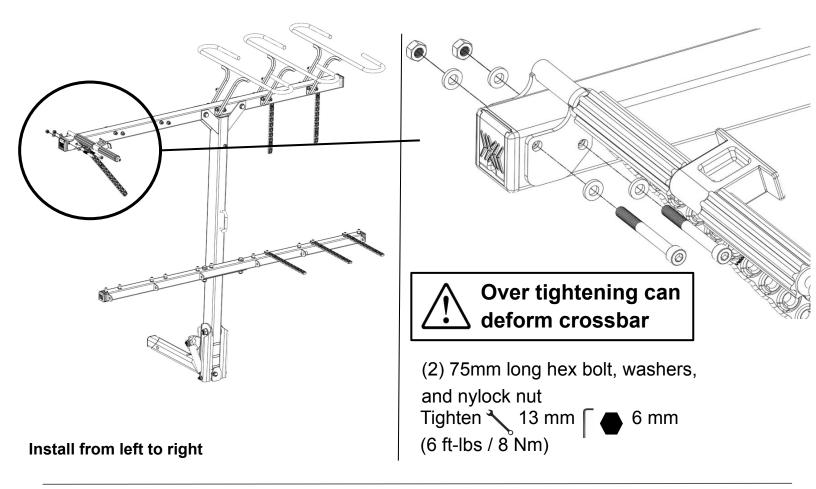
**3.** Slide Bottom Mount Over Anchors and Slide to the Left and Tighten in Place
