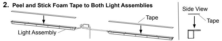
Note: Tape will cover the full surface including the screw holes on the light assembly
