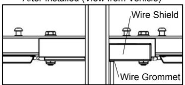
D. Re-tighten both bolts to secure lower bar and wire shield making sure wires
