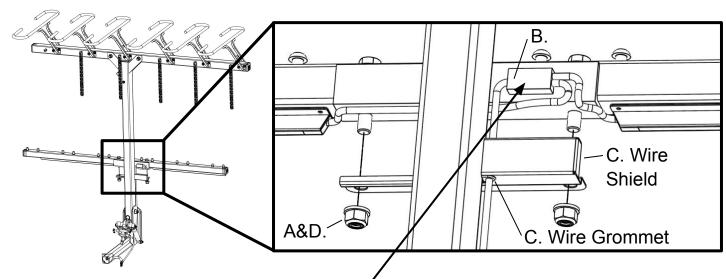
A. Remove 2 nuts securing the lower bar (Do not remove the lower bar)
