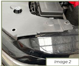
Remove the 2 Oem bolts shown and retain the grey bolt securing the headlight for later use.
