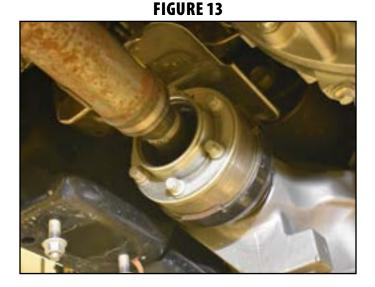
26. **Optional:** Remove the passengers side CV only. Strike the shaft with a hammer to dislodge it from the splines. This will make handling the differential much easier (Fig 14).
