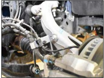
11. Disconnect the tie rod ends from the steering knuckles. Remove and save the nuts. Avoid hitting the aluminum steering knuckle, use appropriate tool to remove tie rod end from steering knuckle. Take care not to strike the tie rod end, or damage the threads (Fig 5). *Note: Use a tie rod end separator to release the taper from the steering knuckle.*
