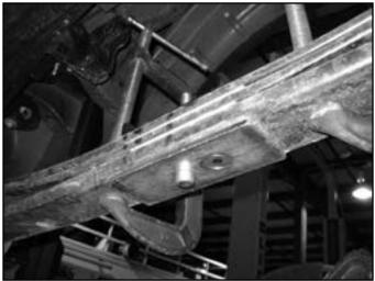
83. Install the new provided lift block so that the bump stop wing goes toward the inside of the vehicle. The block will use the both of the lower center pin holes. The upper only uses 1 hole which will shift the axle slightly forward.
