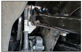
67. Install the supplied 1/4" drive shaft spacer and reattach front drive shaft to differential with new hardware and using the factory washer plates and thread locker (Bolt Pack #828). Torque bolts to 41 ft-lbs (Fig 35).
