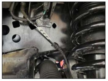
65. Remove the ride height sensor bracket from the upper control arm and disconnect the nut holding the sensor linkage to the bracket. (Fig 33.) Retain hardware.
