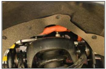
16. Remove the 4 bolts attaching the 4wd actuator hub assembly to the steering knuckle. Figure 9 is shown with the CV shaft pulled out for clarity. Note that some models starting in 2022 will not have the 4wd actuator hub assembly, skid this step if not equipped.
