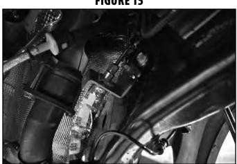
28. Reattach the brake line to the the axle with factory bolts and locations, tighten to 15 ft-lbs.
