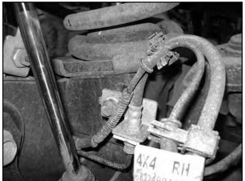
9. It is recommended to disconnect the drag link from the pitman arm at this time. This will prevent the joint from binding while installing new coils. Use care not to damage the drag link joint boot. (Fig 6)
