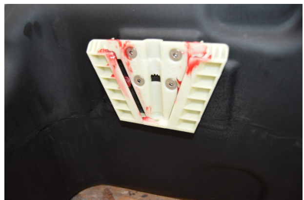
(Fig. 8) It is a good practice to apply a small amount of grease to the water separator mounting bracket to aid in installation of the separator.
