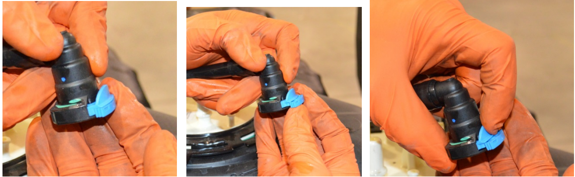
(Fig. 9): Method for Disconnecting Fuel Line Couplings: The majority of the couplings involved in this installation are of the quick connect type shown in left photo above. To disconnect, a) Slide the tab that has teeth on its edge outwards as shown in the center photo. b) Next, press the rounded button, as shown in the right photo, and pull the coupling apart.
