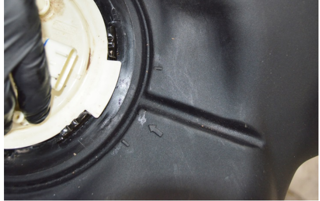
(Fig. 13) Line the tab on the sending unit up with the tab location arrow on the TITAN tank.
