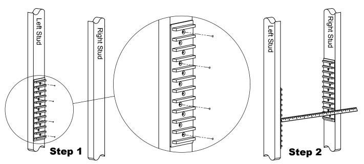
Attach first EZStudRack with 4 supplied screws.
