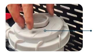
After replacing the filter element. Screw on the filter cover, open the ball valves. Then open the exhaust valve slightly to ensure there are no air locks. After this you can turn the lce bath back on
