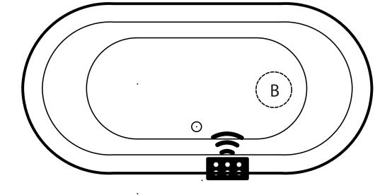
Airbath System III Blower must be remotely located (Diagram is required for custom blower connection locations)
