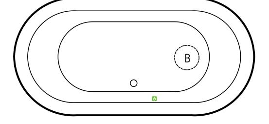
Airbath System III Blower must be remotely located (Diagram is required for custom blower connection locations)
